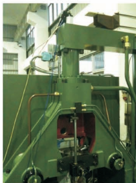
Hot chamber die-cast machine used Germanjet 17 series
