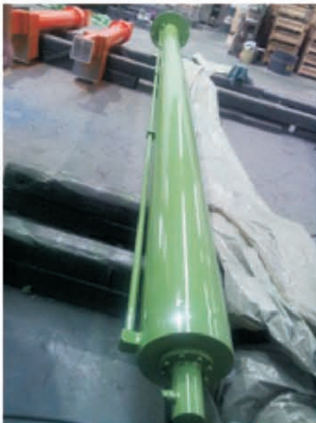
6550mm hydraulic cylinder uses 19 series
