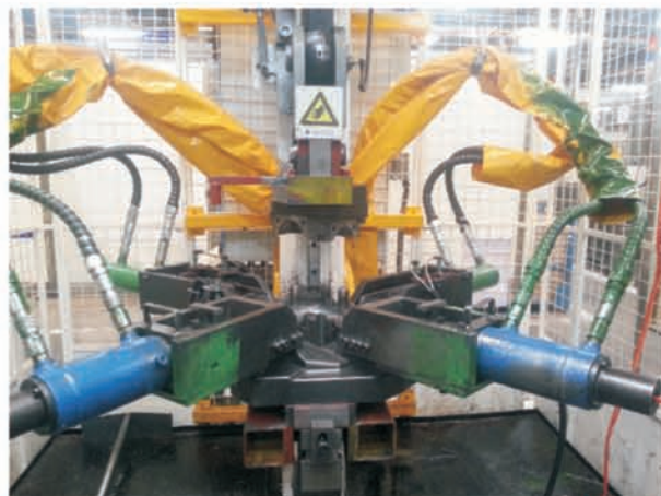
Automotive exhaust pipe bending machine used Germanjet 17 series
