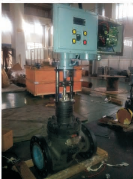
Automatic Control Valve use 17 series
